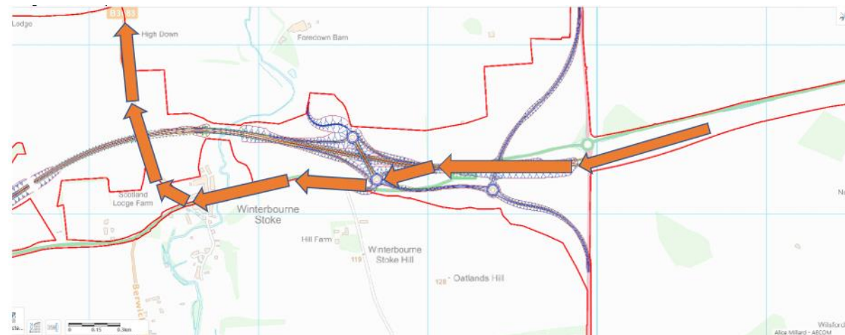
Figure 1: East to North movement on A303 to B3083 through Longbarrow junction for tunnel extension alternatives
